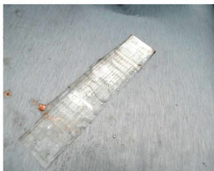
Adhesive strips should be removed from the zinc Surface as soon as detected, and any adhesive residue cleaned.
